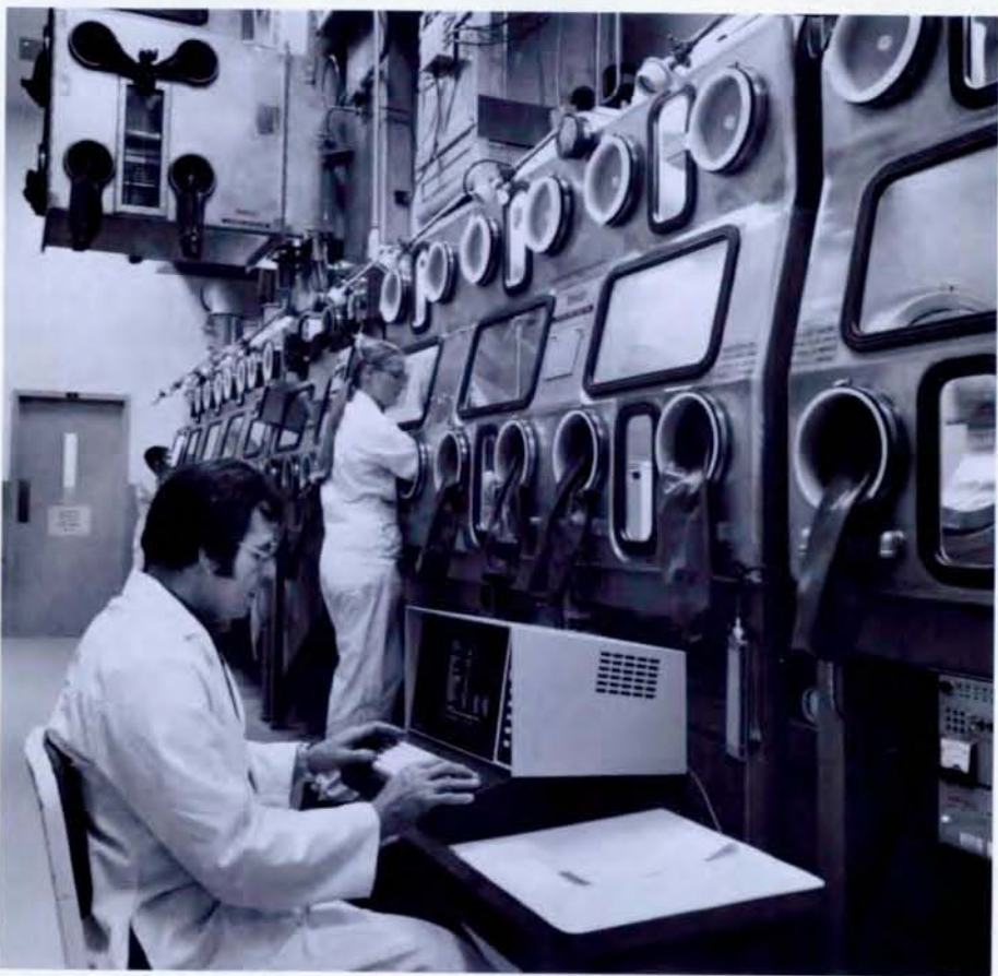
The current Los Alamos plutonium research and development facility. Note, in contrast to the wartime laboratory, the absence of external ventilation on the large research building to the right (upper photograph). The facility uses the most modern equipment, including a computerized plutonium accountability system (lower photograph).
